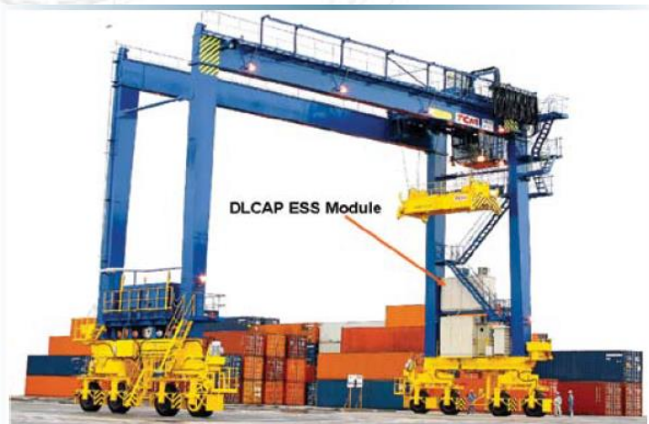
Fig. 1. Hybrid diesel/electric rubber tired gantry crane with an electrochemical capacitor energy storage system. This crane is used for loading and unloading container ships. The capacitor system captures and stores regenerative energy during load lowering that is then used to help raise the next load, resulting in improved efficiency and greatly reduces air emissions. (Photo courtesy of Nippon Chemi-Con Corporation.)
