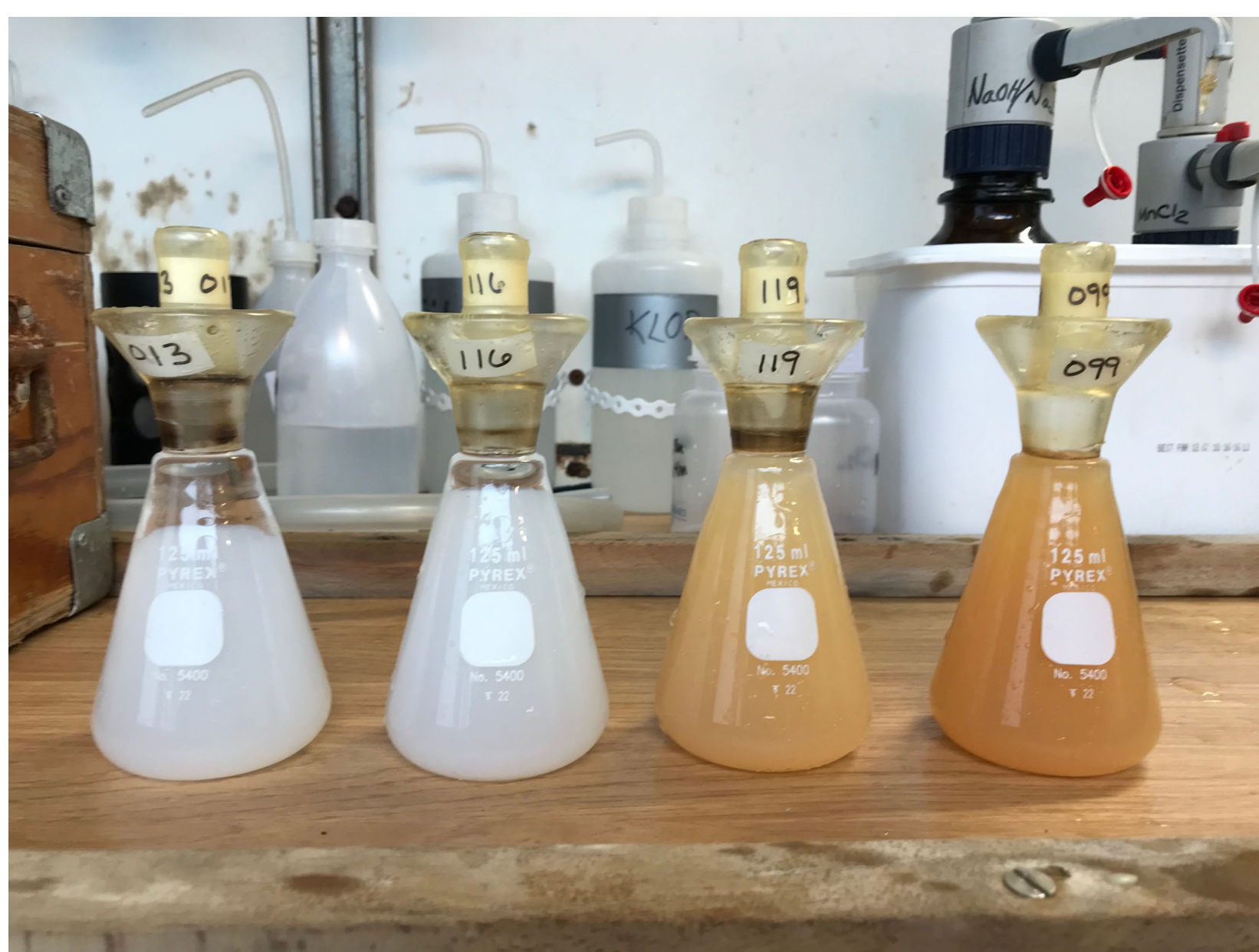
Masfjorden water samples from Cruise KB2022614, with varying levels of dissolved oxygen, increasing from left to right. Photo credits: João Bettencourt.
