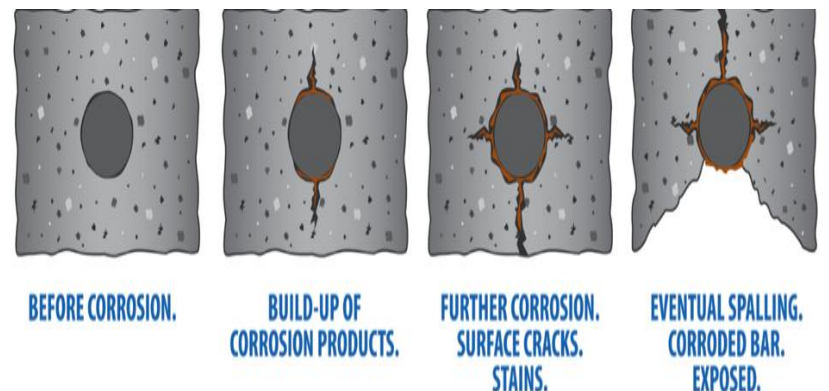
Corrosion cycle of steel.
