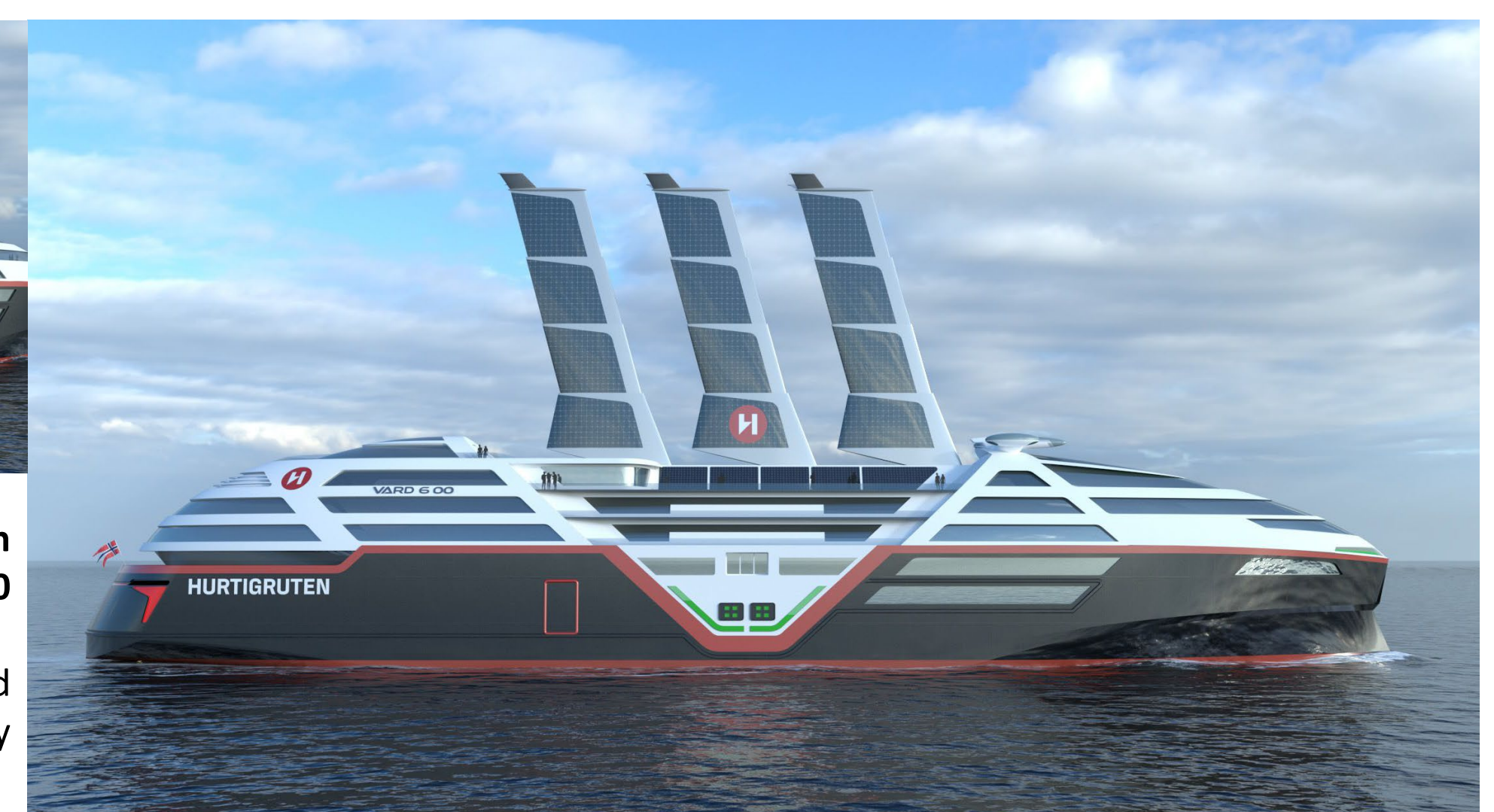
Several companies have started to implement the concept of sailing ships to uses sails mounted on masts to harness the power of wind and propel the vessels. Ayro Ocean Wings is one of them Inspired by the aeroplane wing profiles. Wing-sail system enables new build or existing ships to significantly reduce their fuel consumption.
