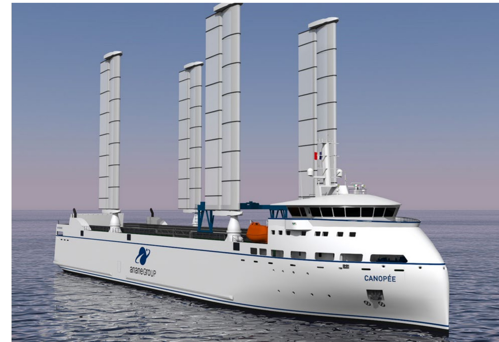
Several companies have started to implement the concept of sailing ships to uses sails mounted on masts to harness the power of wind and propel the vessels. Ayro Ocean Wings is one of them Inspired by the aeroplane wing profiles. Wing-sail system enables new build or existing ships to significantly reduce their fuel consumption.
