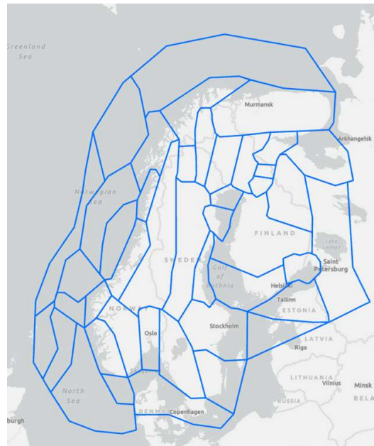
The seismic source zonation model to be used in the baseline probabilistic seismic hazard model for Norway.
