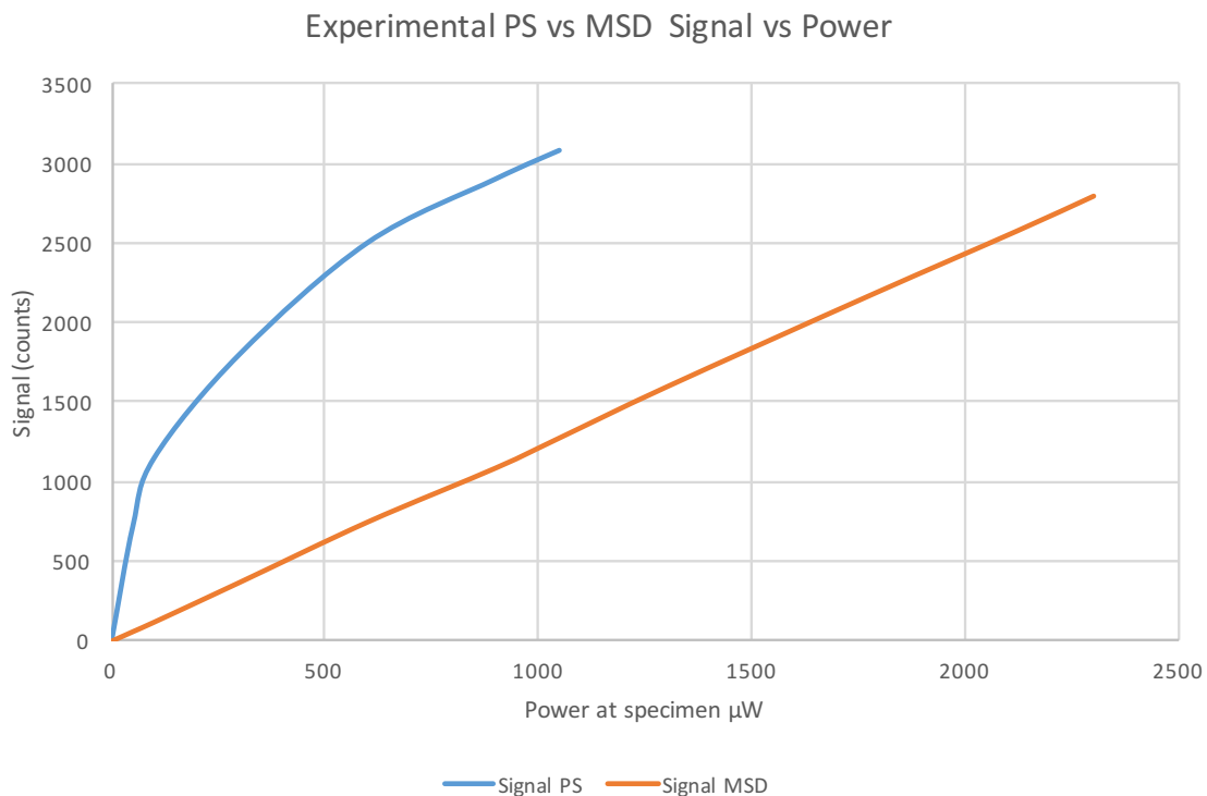
Figure 8. Signal to Power relationship of point scanner (PS) versus microlens spinning disk (MSD) confocal (after Wang et al 2005) with Andor iXon 897 EMCCD camera. Dragonfly uses a unique microlens dual spinning disk design, operating on the same principle as the unit compared by Wang, but with enhanced performance in terms of throughput, field of view and resolution.
