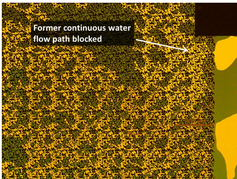
Figure 40: Oil has advanced to block the continuous water flow path observed in Figure 39 as a result of an increased injection rate. Previously trapped water has also been mobilized and displaced.
