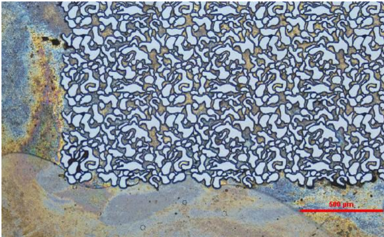
Figure 20: Water filling the channel before entering the matrix.
