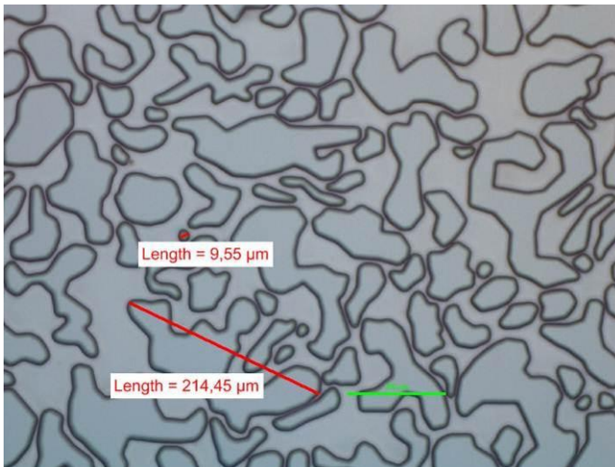
Figure 14: Image taken at 20x magnification of Berea D where grain surfaces are smooth. Both the largest and the smallest grains of the design are captured.
