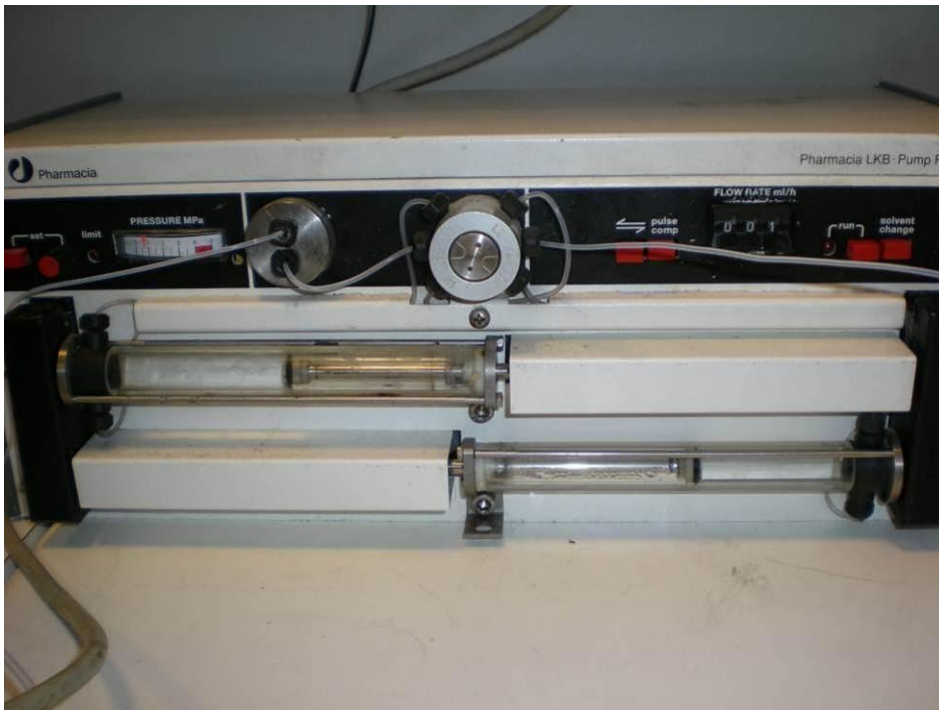
Figure 6: Pharmacia LKB P-500 syringe pump with two syringes.
