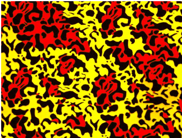
Figure 35: Color thresholding for calculation of fluid saturations in an area swept by oil.
