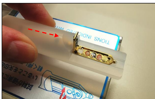
Pull the silicon cylinder to close the metal lid
