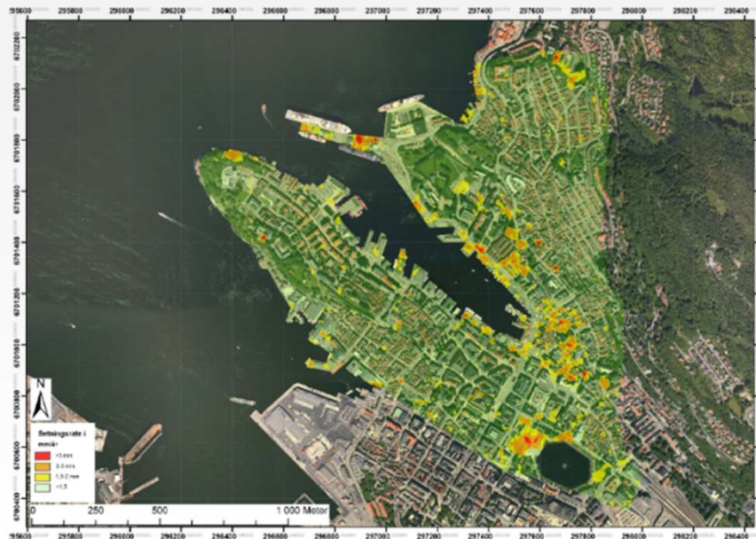
Susceptibility map showing areas in Bergen that are subsiding. Data from InSAR. Made by former masterstudent Joakim Haukedal, 2017.
