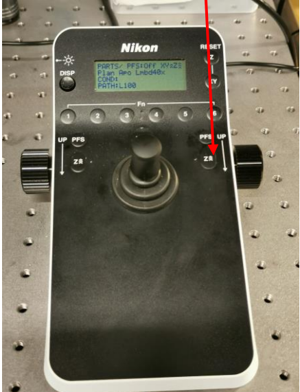
To change the XY speed, press here
