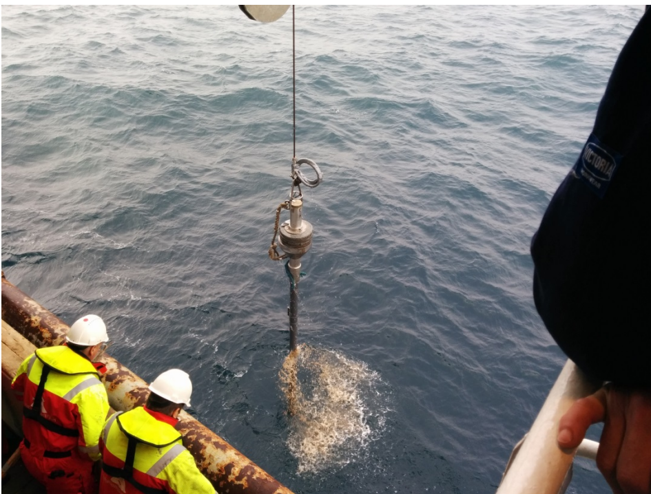
Launching a gravity corer to retrieve ocean floor sediments
