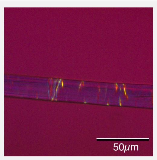
Above: Result of Herzog test showing blue colour in 0°- position and yellow/red in 90°- position.
