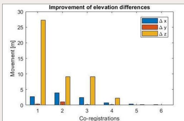
Figure 2. Improvement after co-registration 6 times. Elevation difference is the  $\Delta z$  value.
