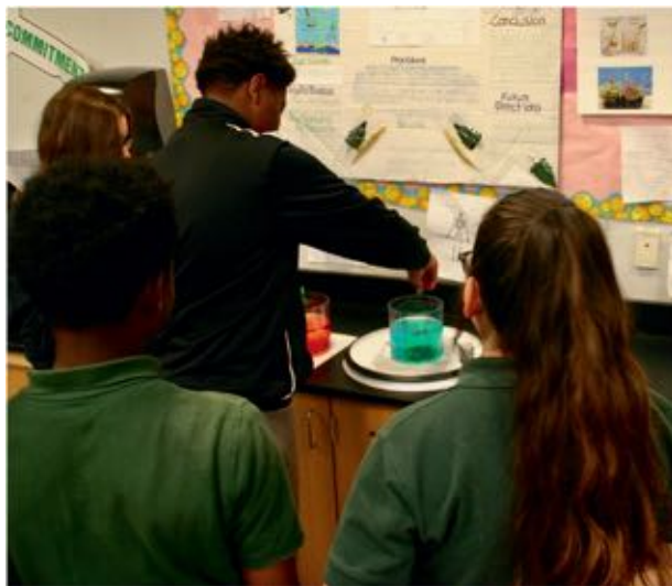
FIG. 4. A student at La Tijera K-8 Charter School in Inglewood, California drops dye into water spinning on the DIYdynamics table as part of a demonstration comparing the behavior of dye in rotating and nonrotating tanks.
