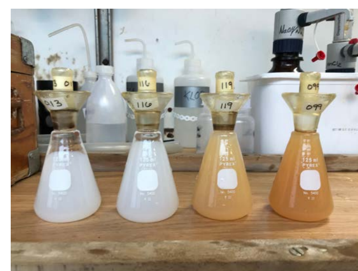
Water samples from Cruise KB2022614, with varying levels of dissolved oxygen, increasing from left to right. May 2022
