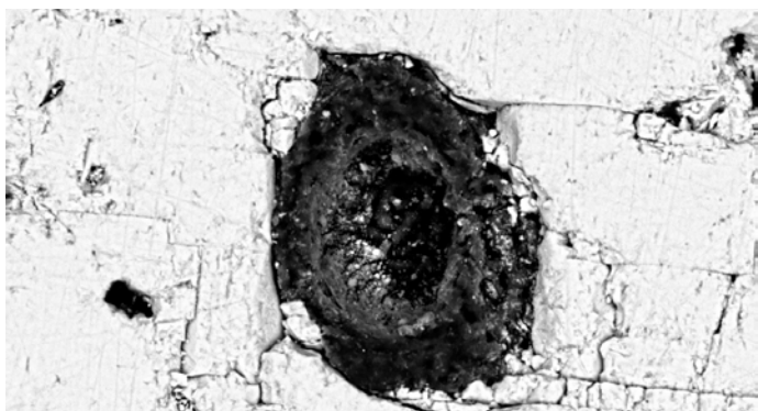
Rounded structures observed from a thin section viewed using an SEM. Could this indicate the past presence of micro-organisms that were degraded and/or later covered by further calcite precipitation?
