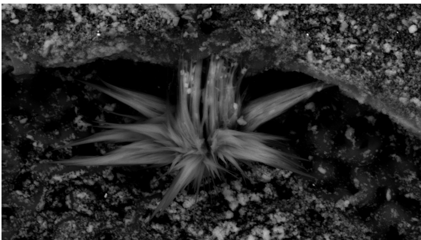
Flower-like structure observed from a thin section using an SEM. This could be a salt crystal.
