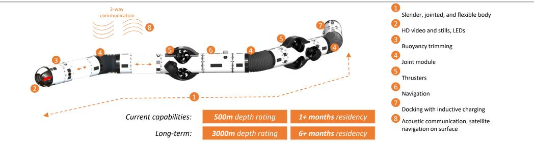
The Eelume vehicle is an *autonomous* underwater *instrument and sensor carrier*: It can connect to a range of different *tools and payloads* to carry out *inspection, survey* and *light intervention* missions in constrained spaces and open waters
