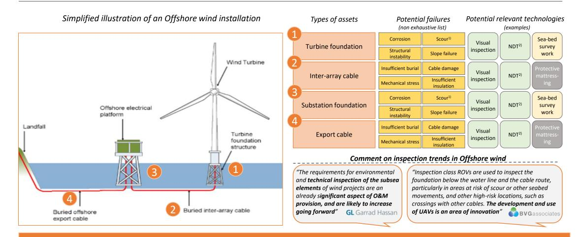
Visual inspection and NDT is key inspection techniques for all Offshore wind subsea installations, and is well suited for Eelume
