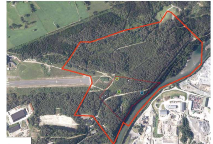
Recommended protection zones surrounding the water works at Bømoen, Voss, a new reserve water supply for Voss municipality. Map made by former masterstudent Line Haukanes, 2018.
