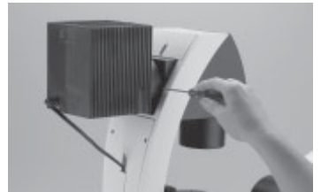
Fig. 49 Connecting the lamp housing to the Leica CTR6000 electronics box
