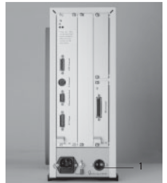
Fig. 49 Connecting the lamp housing to the Leica CTR6000 electronics box
