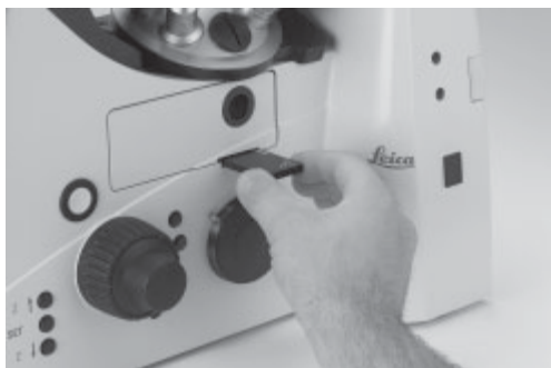
Fig. 110 Inserting the analyzer
