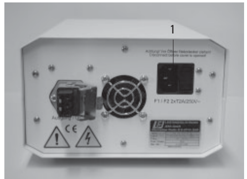
Fig. 79 Rear panel of ebq 100 supply unit 1 AC power socket
