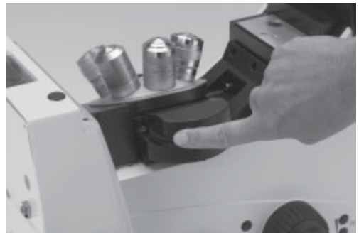
Fig. 111 DIC disk with knurled wheel for fine adjustment
