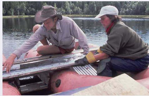
extruding the core
