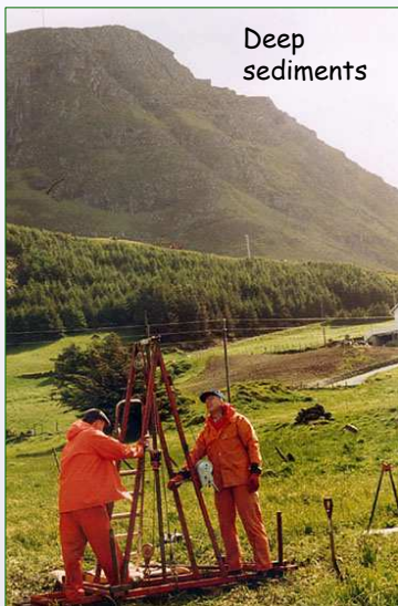
11 cm diameter, 2 m long, piston corer and heavy frame; Kråkenes
