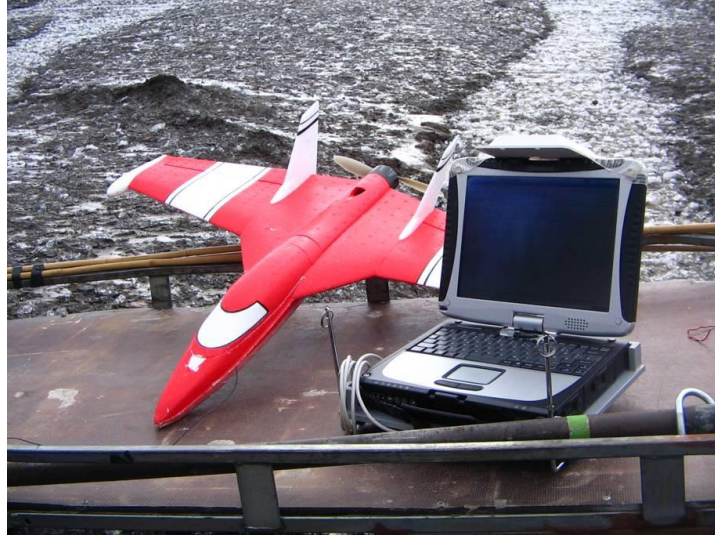
Figure 2: The SUMO airframe and the laptop used as the ground control station.
