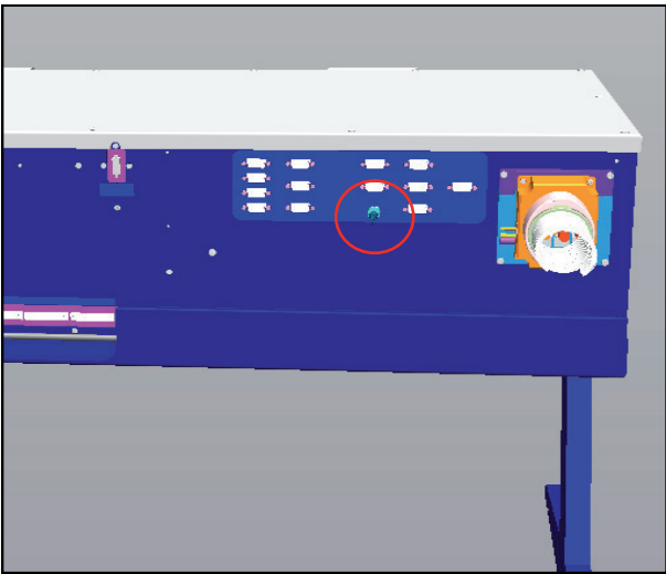
Figure 9: Position of the remote interlock connector
